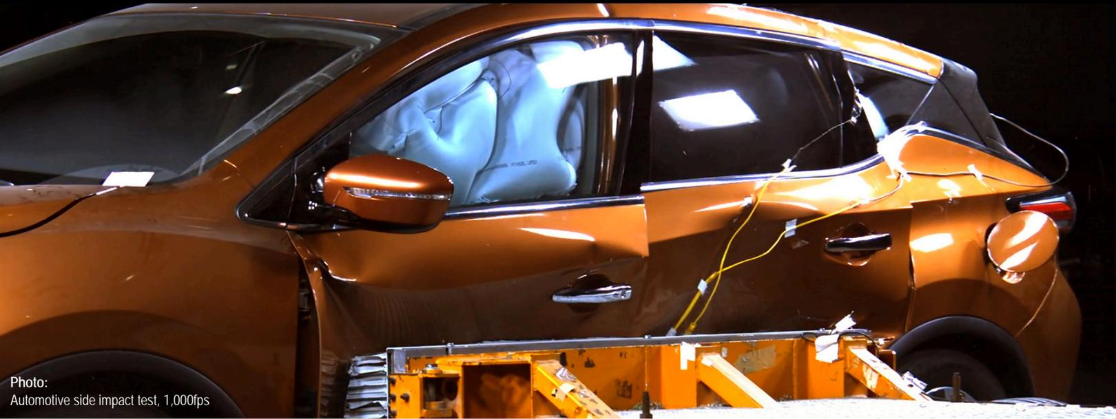
Photo: Automotive side impact test, 1,000fps
