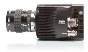
The Os-series is a new digital high-speed camera designed to operate in the most demanding environments. The salient design feature of the Os 7 are its compact size combined with a wide data bus, making it capable of achieving very high frame rates (up to 2,700 fps) including transfer speeds to high-capacity solid-state (non-volatile) memory. Configurable DDR options include 8GB, 16GB, and 32GB.
